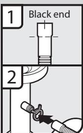
1. Connect black end of of drain hose to waste tee and cut if needed.
